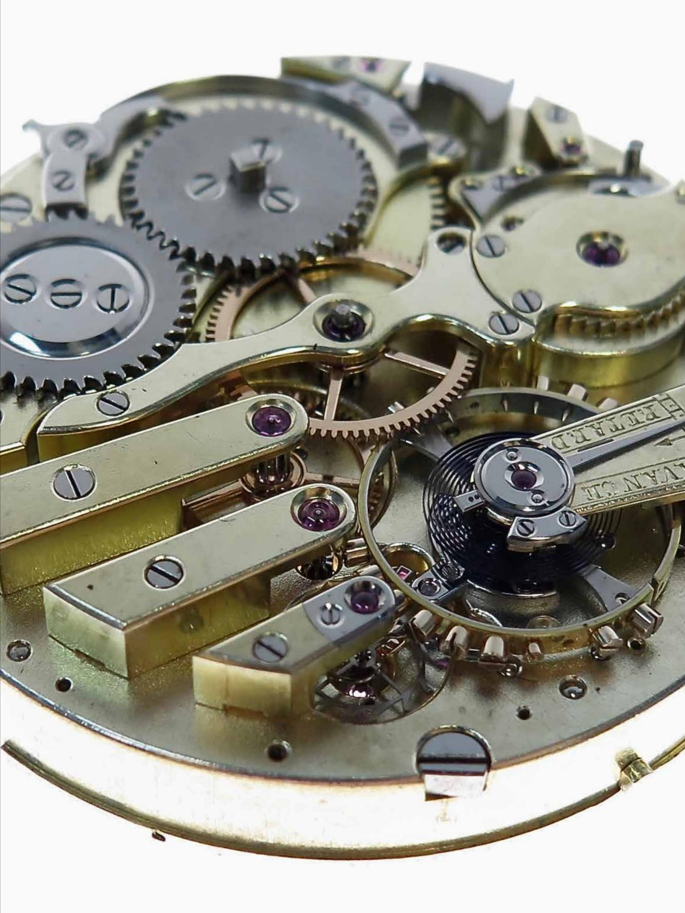
The bridge side of the movement once removed from the case. The repeater sits built into the movement. The calendar mechanism is modular but still sits flush into the movement mainplate.
